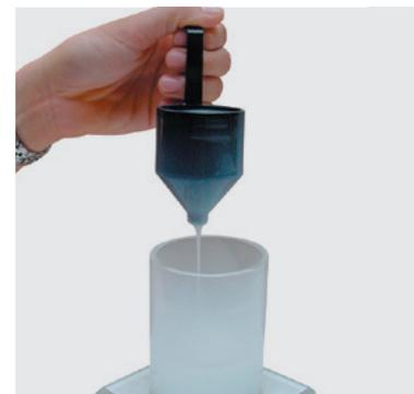
Viscosity testing device
